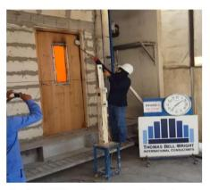
Ramkor FD90™ repeatedly over performs when tested to BS 476 (average result is in excess of 100 minutes fire resistance)
